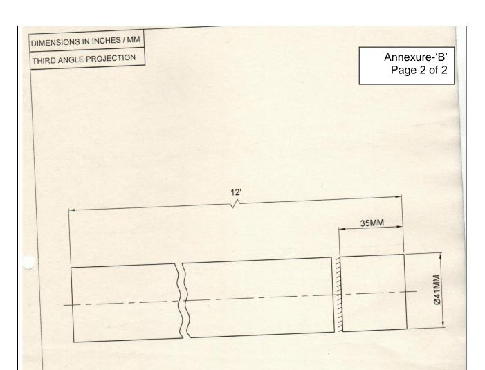
BRASS TO SPEC. BS 2874, CZ-121 4Pb (FOR FREE MACHINING)
