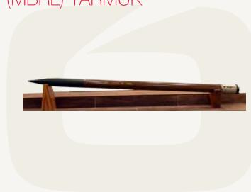
Rocket 122mm HE (MBRL) is a ground to ground free flight artillery rocket fired from multitube launcher. It is used against personnel and light materials providing both fragmentation and blast effect.
